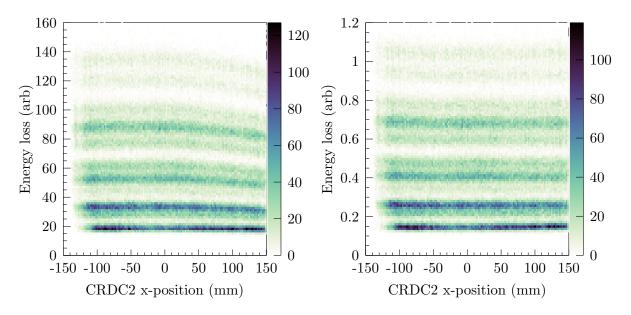
Figure 4.8: Position dependence of the ion chamber. The left panel shows the summed signal from the ion chamber as a function of CRDC2 x-position when using a cocktail beam. The right panel shows the position-corrected summed signal from the ion chamber.
