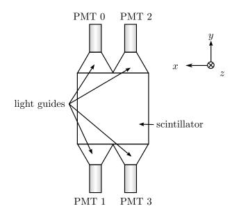
Figure 3.5: A schematic of the thin scintillator, as seen from upstream of the detector.
