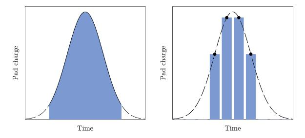
Figure 4.2: Example charge distribution on CRDC pads as a function of time. A full charge integration measurement would integrate the shaded area on the left. The sampling method adds the values of a discrete number of points, as shown on the right.
