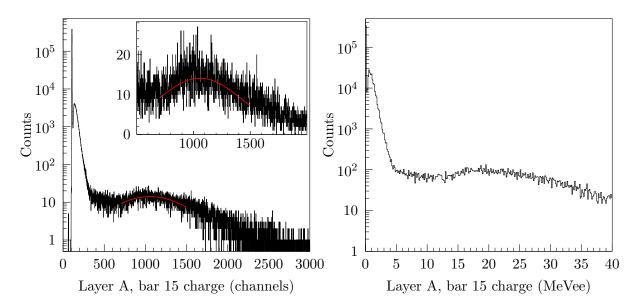
Figure 4.14: An example of MoNA-LISA's charge calibration procedure. The raw charge from each QDC channel is plotted (left). The cosmic peak around channel 1200 is fit with a red Gaussian line. The inset shows channels 500 to 2000 with a linear scale on the y-axis. Those values are used to construct a linear fit whose slope and offset are applied to produce a calibrated charge signal in MeVee (right).
