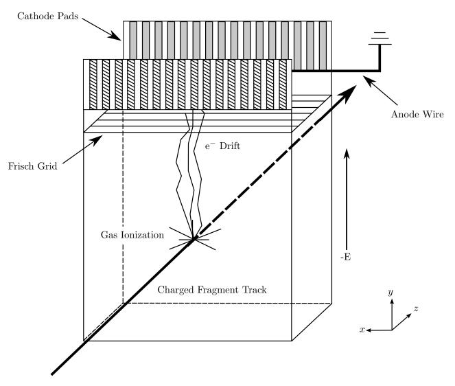
Figure 3.3: Schematic of CRDC operation modified from [139] where the z-direction has been expanded for detail. The field shaping wires mentioned in the text are not included for visibility and simplicity.
