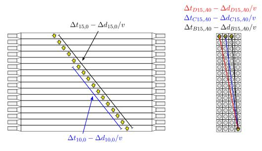
Figure 4.18: Schematics showing the differences used to calibrate the time measurement in MoNA-LISA. The view on the left is from the front of the array and the schematic on the right shows the side view of the array, looking head-on at the PMTs.
