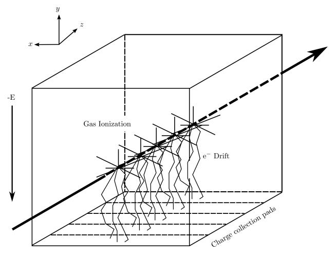
Figure 3.4: Schematic of ion chamber.
