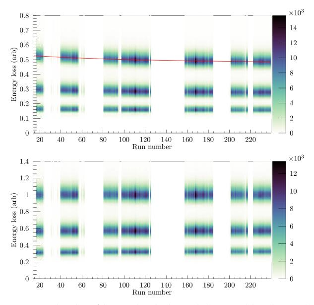
Figure 4.9: Time dependence of the summed ion chamber signal. The top panel shows the summed, position-corrected ion chamber signal as a function of run number. The red line is the fitted function 4.3 using parameters from Table 4.3. The bottom panel shows the summed, position-corrected, and time-corrected ion chamber signal as a function of run number.
