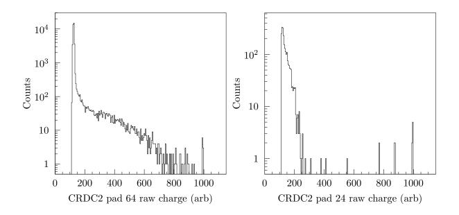
Figure 4.1: Examples of total charge spectra for two pads in CRDC2. Pad 64 (left) is an example of a good total charge spectrum and pad 24 (right) is an example of a bad total charge spectrum.
