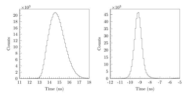
Figure 4.12: Timing signal from the target scintillator before (left) and after (right) the walk correction.
