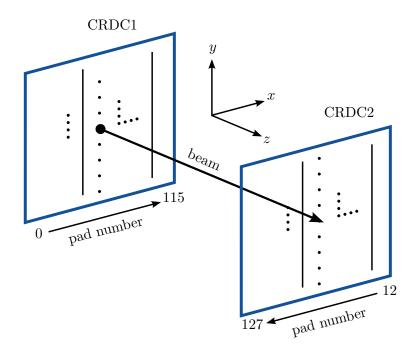
Figure 4.6: A schematic of the CRDC masks and their relation to the lab coordinate frame, the beam, and the pads in each detector.
