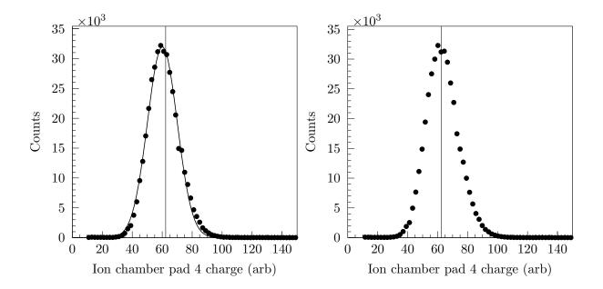
Figure 4.7: An example of fitting used in gain-matching the ion chamber. Left: points show raw charge signal from pad 4, thick solid line is Gaussian fit to data, and thin vertical line indicates centroid of "ideal" pad 8. Right: points show gain-matched charge signal from pad 4 and thin vertical line indicates centroid of "ideal" pad 8.
