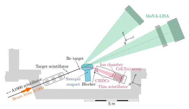
Figure 3.2: Schematic of the experimental area.
