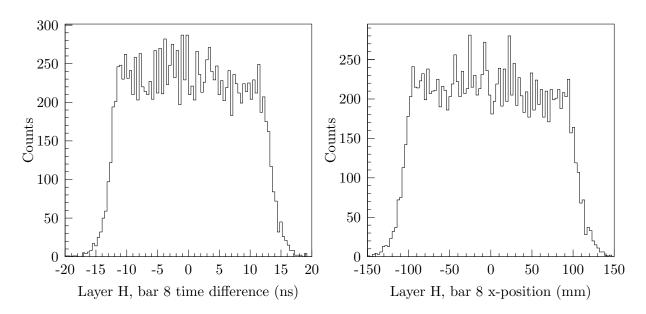
Figure 4.17: X-position calibration example. The final x-position spectrum (right) for one bar was calculated based on the time difference between the two PMTs (left).
