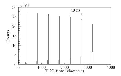
Figure 4.15: An example of the raw time spectrum during MoNA-LISA's TDC calibration procedure. A pulser pulses the system every 40 ns, creating a spectrum with peaks at intervals that correspond to 40 ns.
