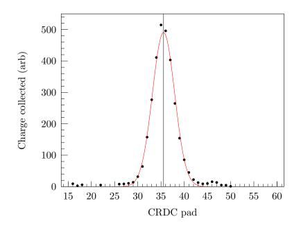
Figure 4.4: An example of a charge distribution fit for CRDC2. The centroid of the Gaussian fit, shown here by the vertical line, would be used as the position of the particle in this detector.
