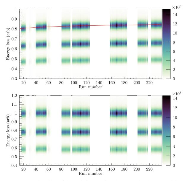
Figure 4.11: Time dependence of the total thin scintillator charge signal. The top panel shows the summed, position-corrected thin scintillator charge signal as a function of run number. The red line is the fitted function 4.3 using parameters from Table 4.5. The bottom panel shows the summed, position-corrected, and time-corrected charge signal as a function of run number.
