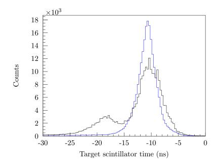
Figure 4.13: Target scintillator timing spectra from run 41 (black), taken while the target exhibited double peaking, and from run 90 (blue), taken after the double peaking was fixed.
