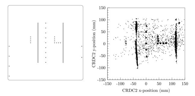
Figure 4.5: Left: mechanical design drawing of the CRDC mask. Right: Example of CRDC mask data from run 157.
