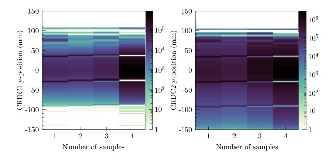
Figure 4.3: CRDC *y*-position versus number of samples collected for each pad (left: CRDC1, right: CRDC2). Both plots are shown with the z-axis on a log scale. Each CRDC collects fewer samples at certain regularly spaced intervals along the y-direction, visible in these plots as enhancements at lower numbers of samples and vacancies at the spectra for four samples.
