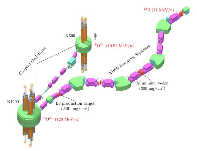
Figure 3.1: Schematic of the Coupled Cyclotron Facility and A1900 Fragment Separator with the production setting for this experiment.
