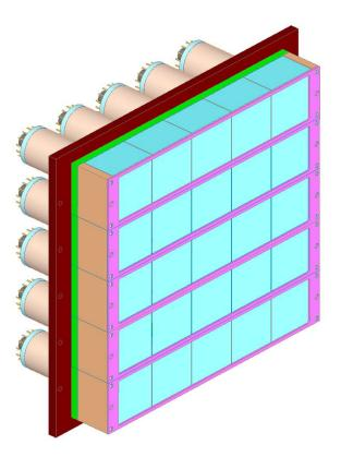
Figure 3.6: A mechanical design drawing of the CsI(Na) array.
