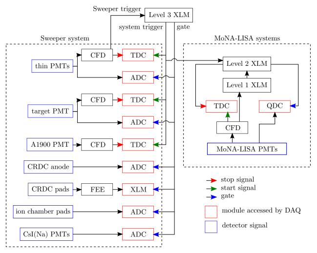
Figure 3.8: Schematic of the MoNA-LISA-Sweeper electronics set-up.
